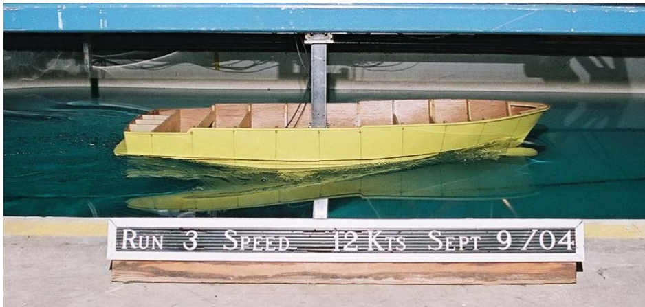
Model testing an 86 ft. motoryacht with a bulbous bow.
