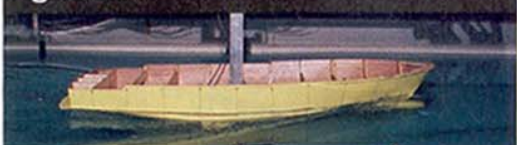
Tank tests at the Ocean Engineering Centre, University of British Columbia. Fig. 6a —A typical trawler hull at 10 knots. 6b —The Fox 86 at 10 knots. 6c —Typical trawler at 13 knots. 6d —Fox 86 at 13 knots.
